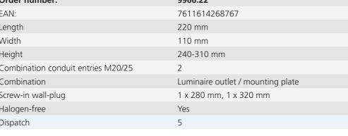
The system equipment carrier is designed to fit perfectly into the external insulation and in this way reliably prevents heat bridges. Easy, fast fixing with the screw dowles included in the scope of delivery permanently anchors the system equipment carrier on many surfaces. Ideal for stable fixing of external lamps, sockets, door intercom devices and many more. nd permanently. Heavy loads are not a problem.
