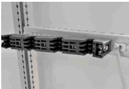
Fix the supports on the crosspieces using M6 screws (tightening torque 10 nm).
