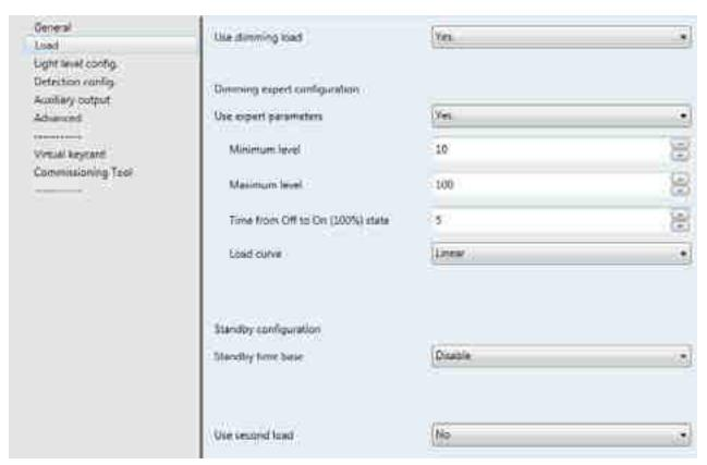
When dimming expert configuration is yes: this object communication is available.
