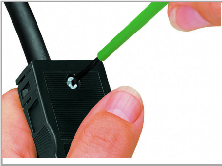
Tighten strain relief screw via screwdriver (2.5 mm blade width).
