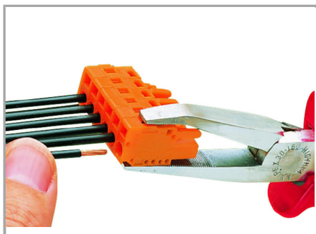
Inserting a conductor via operating tool.
