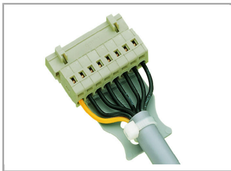
Male connector with strain relief plate
