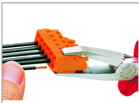
Inserting a conductor via operating tool.
