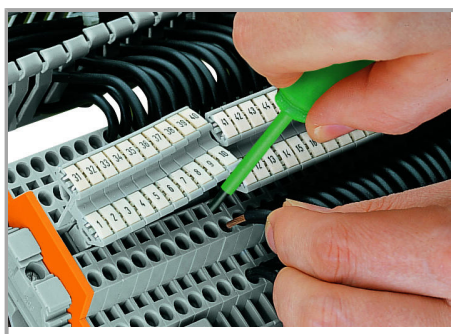
The flexible marker carrier, which is placed above the wiring level, can be pushed aside during wiring or commoning. The carrier has two staggered levels for WMB markers that perfectly align with the terminal block decks.
