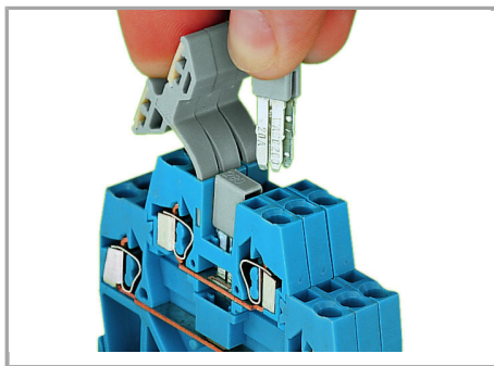
Commoning using an adjacent jumper (280-402).
