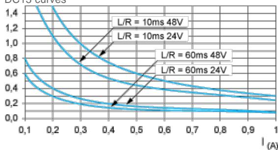
DC13 switching electromagnets,  $L/R \leq 2 \times (U_e \times I_e)$  in ms,  $U_e$ : rated operational voltage,  $I_e$ : rated operational current (with a protective diode on the load, DC12 curves must be used with a coefficient of 0.9 applied to the number in millions of operating cycles)
