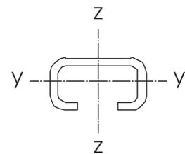
$$\begin{aligned}W_y &= 0.32 \text{ cm}^3 \\W_z &= 0.83 \text{ cm}^3 \\I_y &= 0.30 \text{ cm}^4 \\I_z &= 1.26 \text{ cm}^4\end{aligned}$$
